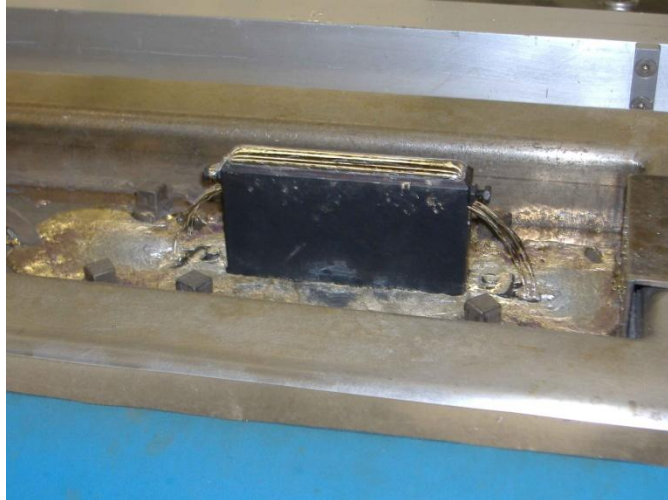
Figure 6.5. Hybrid nozzle during rework operations.
